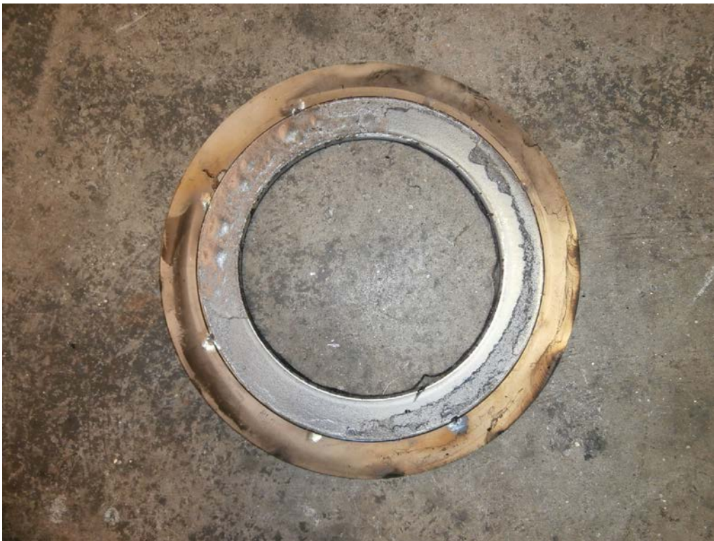
Test Gasket Post-Burn
